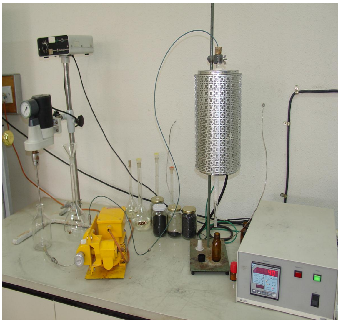
Figure 1: photograph of assembled apparatus used for adsorption.
