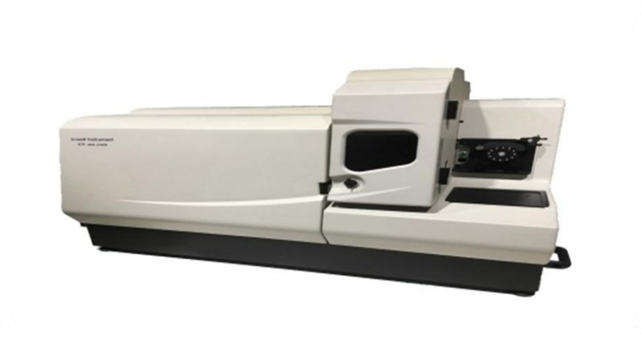
Figure 4: Shown the ICP–MS instrument used the inert argon gas as a plasma source to generate the ionization state for elements of cadmium and lead.
