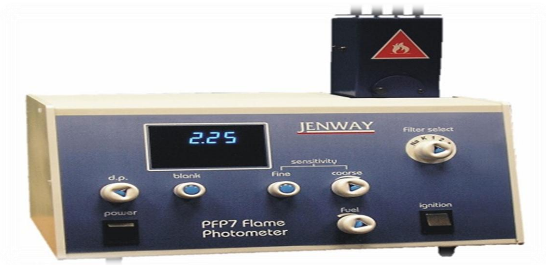
Figure 3: Shown the Jenway flame photometer models PFP7. Where using to determined concentrations of Na and K in seawater samples.
